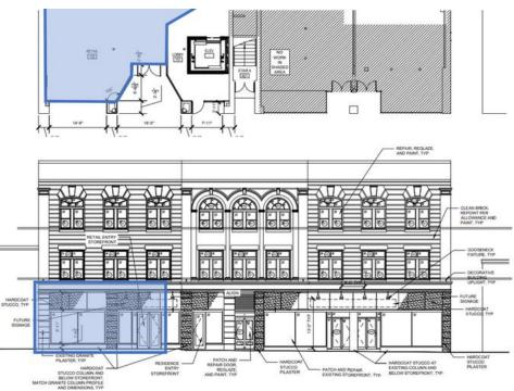
Top: Preliminary floor plan of entrance to space. The remainder of the floor plan is open with a small mezzanine area.
